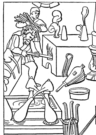
FIG. 1.—DISTILLATION APPARATUS OF ABOUT A D. 1556. IN THE FOREGROUND RETORTS ARE BEING HEATED IN A VESSEL OF WATER, ATTACHED TO RECEIVING FLASKS BY ALEMBCS OR HEADS
